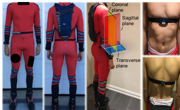
Fig. 1 Location of the seven triaxial IsenseU-Ski sensors and sensor orientation relative to the skier
