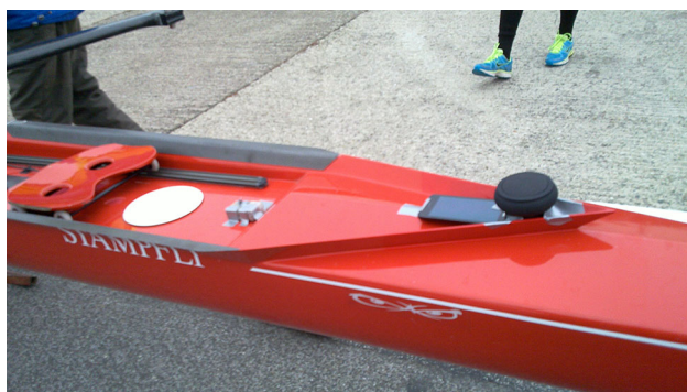
Fig. 2 The equipment used in Experiment 2 consisted in a smartphone running Android OS, one monophonic loudspeaker, and one external accelerometer. Boat acceleration was collected by the smartphone’s internal accelerometer and fed into the sonification model directly, as well as logged by an external accelerometer at a higher sample rate. The auditory feedback was synthesised using the program ScenePlayer running on the smartphone
