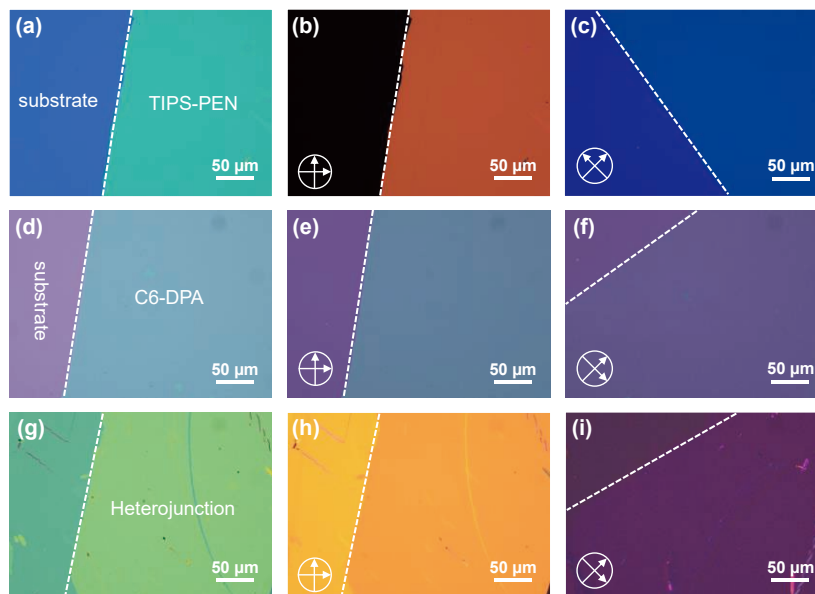
Figure 1 OM images of both 2DMCs and their heterojunctions. OM images of 2DMCs of (a) TIPS-PEN, (d) C6-DPA and (g) their heterojunctions, respectively. (b) and (c) POM images of 2DMCs of TIPS-PEN. (e) and (f) POM images of 2DMCs of C6-DPA. (h) and (i) POM images of heterojunctions.
