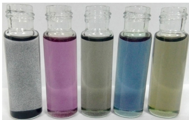
Figure 1 Photographic images of the samples dispersed in DMSO (from left to right: MWCNTs, SnTPP 1, MWCNT-SnTPP 1, SnTPP 2, and MWCNT-SnTPP 2).
