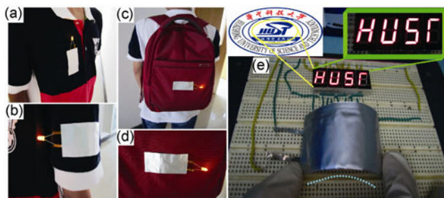
Figure 5 (a)–(d) Optical images of a flexible/ultra-thin Li-ion battery transferred onto daily clothes and travel bag, showing its future wide wearable/portable electronic applications. (e) A flexible lithium-ion battery lighting four Nixie tubes, showing the logo of “HUST”.
