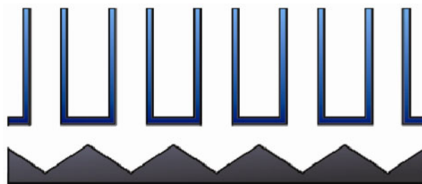
Figure 2 By carefully arranging the locations of the nanowires and tailoring the wet-etching time, it is possible to link neighbouring under-etched areas to create a continuous channel
