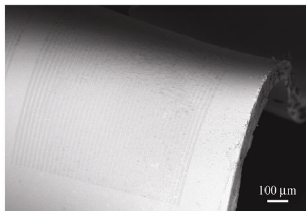
Figure 35 Low magnification SEM image of patterned nanowire arrays transferred onto a flexible substrate [56]. Reproduced with permission
