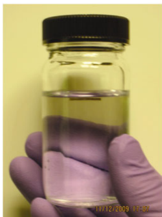
Figure 9 A photograph of the reaction container showing the substrate floating on the solution surface by surface tension
