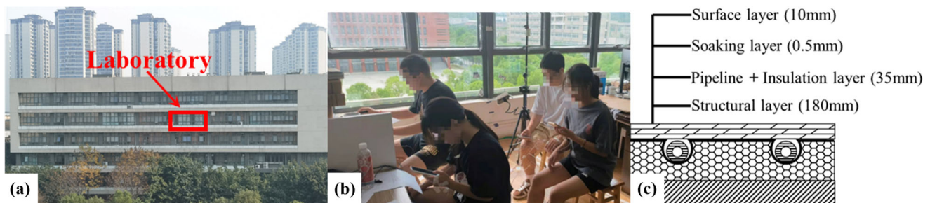
Fig. 2 Laboratory introduction: (a) photo of the laboratory, (b) test image of the subjects, (c) diagram of the radiation terminal structure
