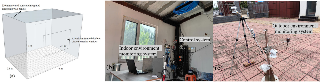
Fig. 9 Laboratory and instrument layout: (a) schematic diagram of laboratory and (b) schematic diagram of the field test in the laboratory
