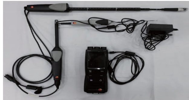
Fig. 7 The thermo-hygrometer sensor "Testo 480"
