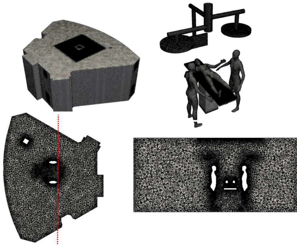
Fig. 3 Computational grid of the OR with real human shapes and other equipment
