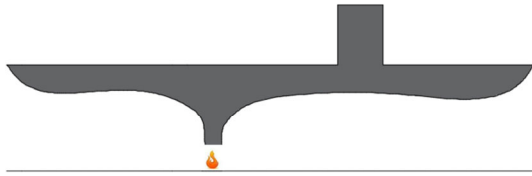
Fig. 2 Schematics of the smoke exhaust in a tunnel fire with a vertical shaft
