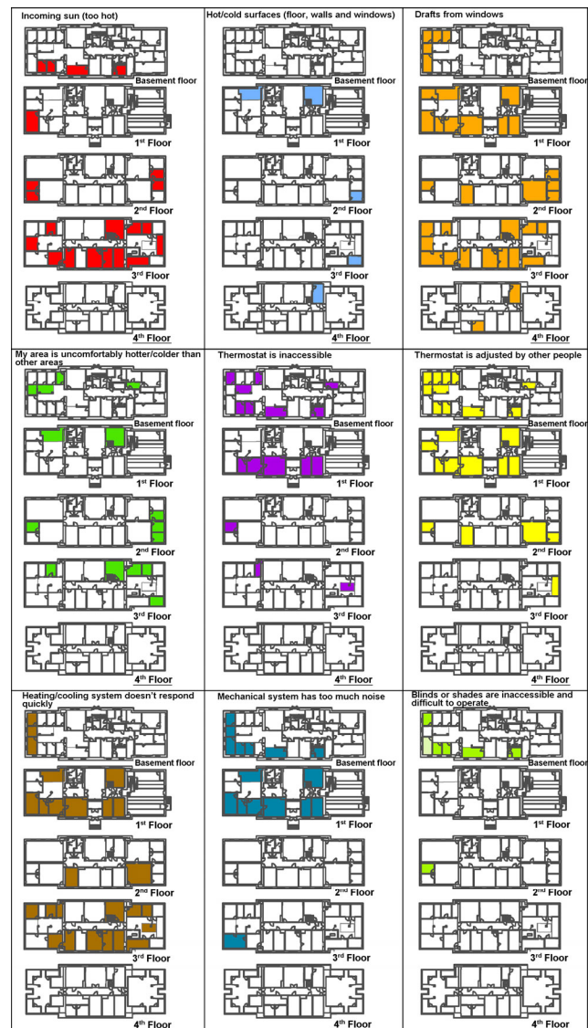
Fig. 9 Spatial mapping of the portable devices for each zone on each floor
