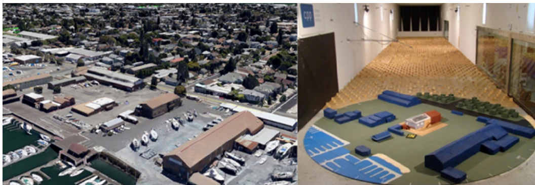
Fig. 1 Aerial view (left), wind tunnel model of the main building and surrounding buildings (right)
