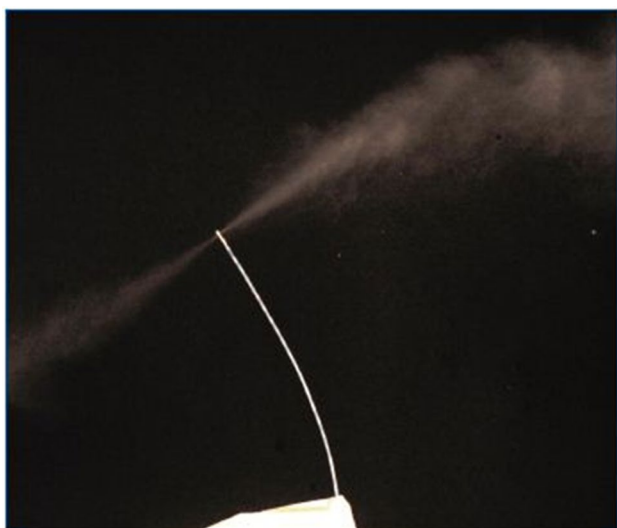
Fig. 7 Steam is ejected from two areas at the tip of the catheter
