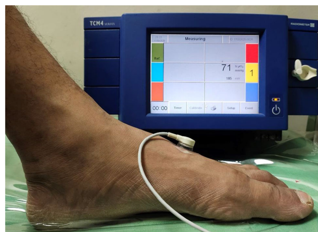
Fig. 1 Recording of TcPO 2 by keeping an adhesive sensor to the foot and monitor displaying value of TcPO 2
