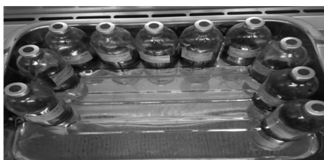
Fig. 2. Batch mode serum bottle experimental set-up (inside a 30°C incubator).
