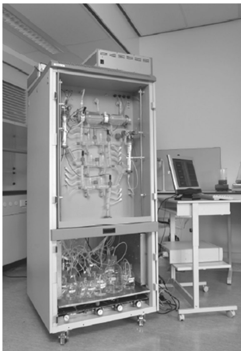
Fig. 3 TNO TIM-1 digestion model device. Reprinted with permission from John Wiley & Sons [3]
