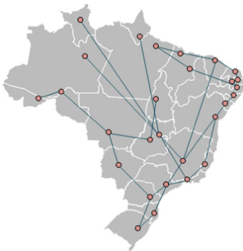
Fig. 10 Brazilian Rede Nacional de Ensino e Pesquisa (RNP) real topology, with 31 vertex and 34 edges
