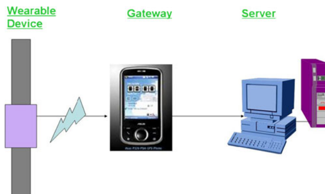
Fig. 3 Three stages of data transfer: acquisition, forwarding and storage
