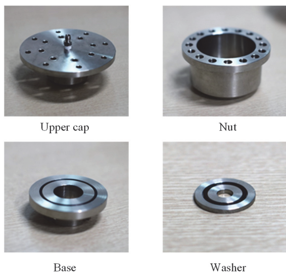
(a) Part of injection equipment
