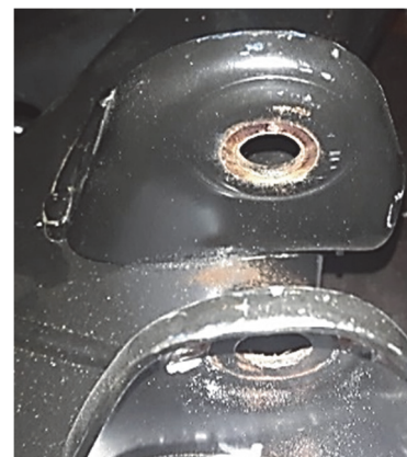
Figure 10. State of the lap surface after fatigue tests.
