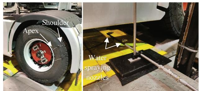
Figure 3. Truck measurement setup with thermocouple temperature sensors drilled into a tyre (left) and water spraying nozzle in front of the tyre (right).
