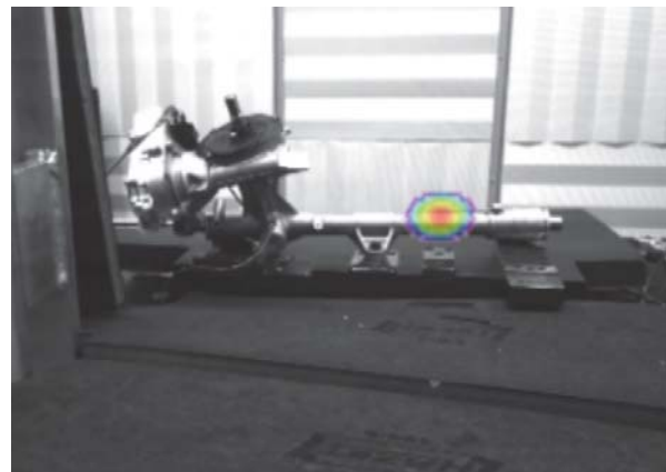
Figure 20. Acoustic photo – Noise localization at 8200 (Hz).
