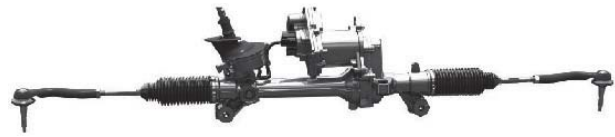
Figure 2. Rack-assist EPS (REPS).
