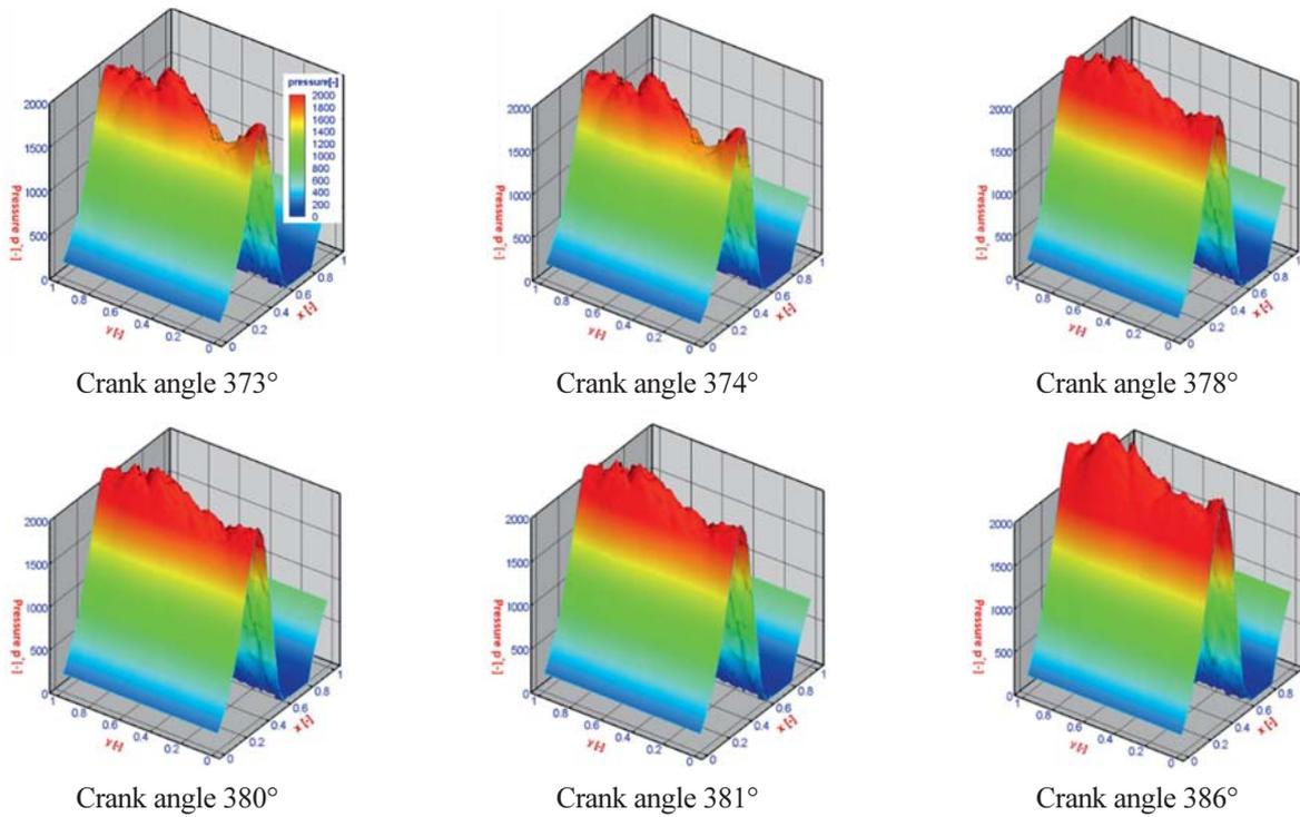
Figure 8. Variations in the hydrodynamic dimensionless pressure  $p^* = (p - p_{atm}) / (\mu U_{cr=1^\circ} l_{pr})$  during a cycle on smooth cylinder surface ( $\mu = 5.5 \text{ mPas}$ ,  $U_{cr=1^\circ} = 0.3174 \text{ m/s}$ ,  $l_{pr} = 1.2 \text{ mm}$ ) at 3000 rpm under full load.
