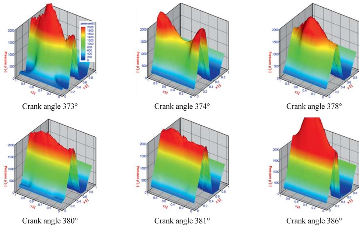
Figure 6. Variations in the hydrodynamic dimensionless pressure  $p^* = (p - p_{atm})/(\mu U_{cr=1^\circ} l_{pr})$  during a cycle on LST cylinder surface ( $\mu = 5.5 \text{ mPas}$ ,  $U_{cr=1^\circ} = 0.3174 \text{ m/s}$ ,  $l_{pr} = 1.2 \text{ mm}$ ) at 3000 rpm under full load.
