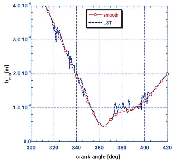
(b) Film thickness selected power stroke crank angle range
