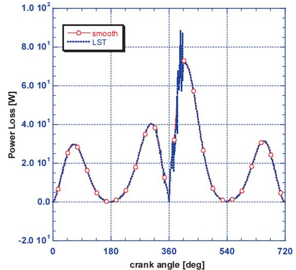
(a) Frictional power loss during a cycle
