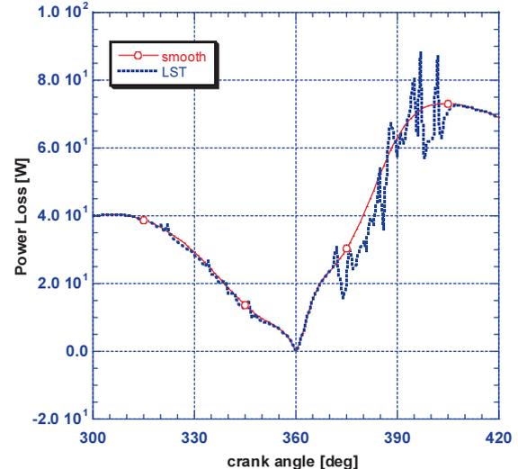
(b) Frictional power loss during selected crank angle range
