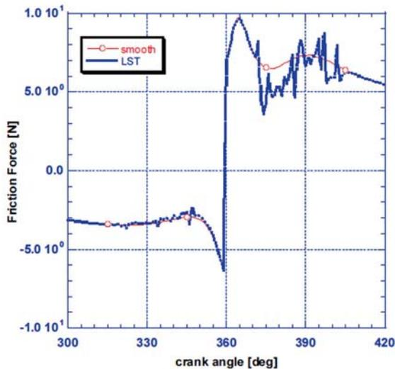
(b) Frictional force during selected crank angle range
