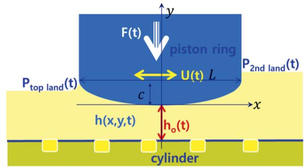
Figure 2. Piston ring profile and boundary conditions for the hydrodynamic lubrication computation with top and second land pressures.
