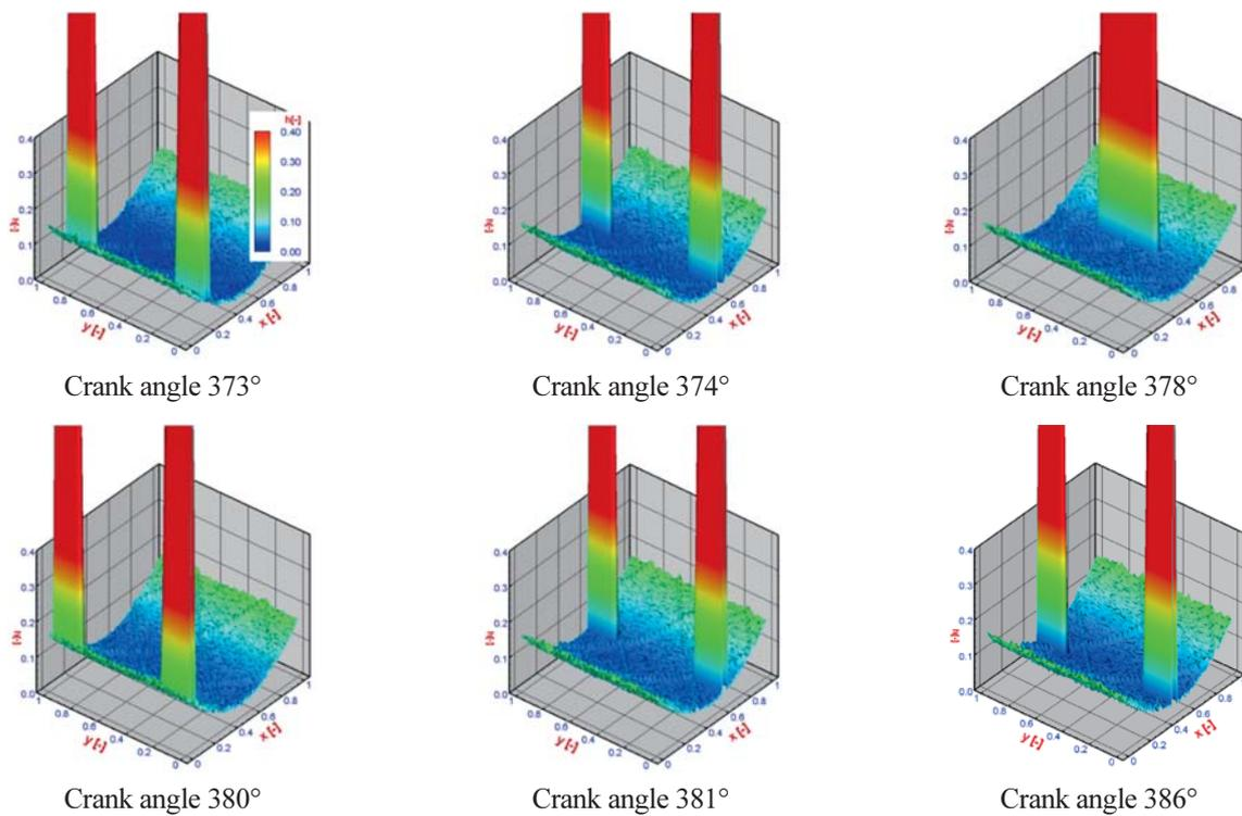
Figure 7. Variations in the hydrodynamic dimensionless lubrication film  $h^* = h/h_{max}$  during a cycle on LST cylinder surface ( $h_{max} = \text{LST depth} + \text{honing ridge depth} + R_a$ ) at 3000 rpm under full load.
