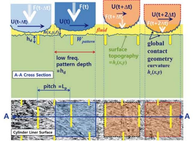
Figure 4. Cylinder liner surface with LST and variation in the contact geometry as the piston ring's stroke from the TDC to BDC (LST depth = 20.0  $\mu\text{m}$ ,  $R_a = 0.3 \mu\text{m}$  honing groove depth = 1.5).
