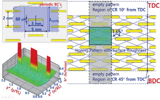
Figure 3. LST pattern at a depth of 20.0  $\mu\text{m}$  on cylinder liner around TDC from crank angle of 10  $\sim$  45 $^\circ$  from TDC and honed surface roughness  $R_a = 0.3 \mu\text{m}$ , honing groove depth = 1.5  $\mu\text{m}$ , honing ridge angle = 45 $^\circ$ .
