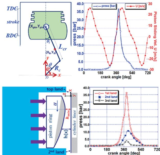
Figure 1. Piston's primary movement in the cylinder liner and piston ring's applied load by combustion pressure at 3000 rpm under full load.
