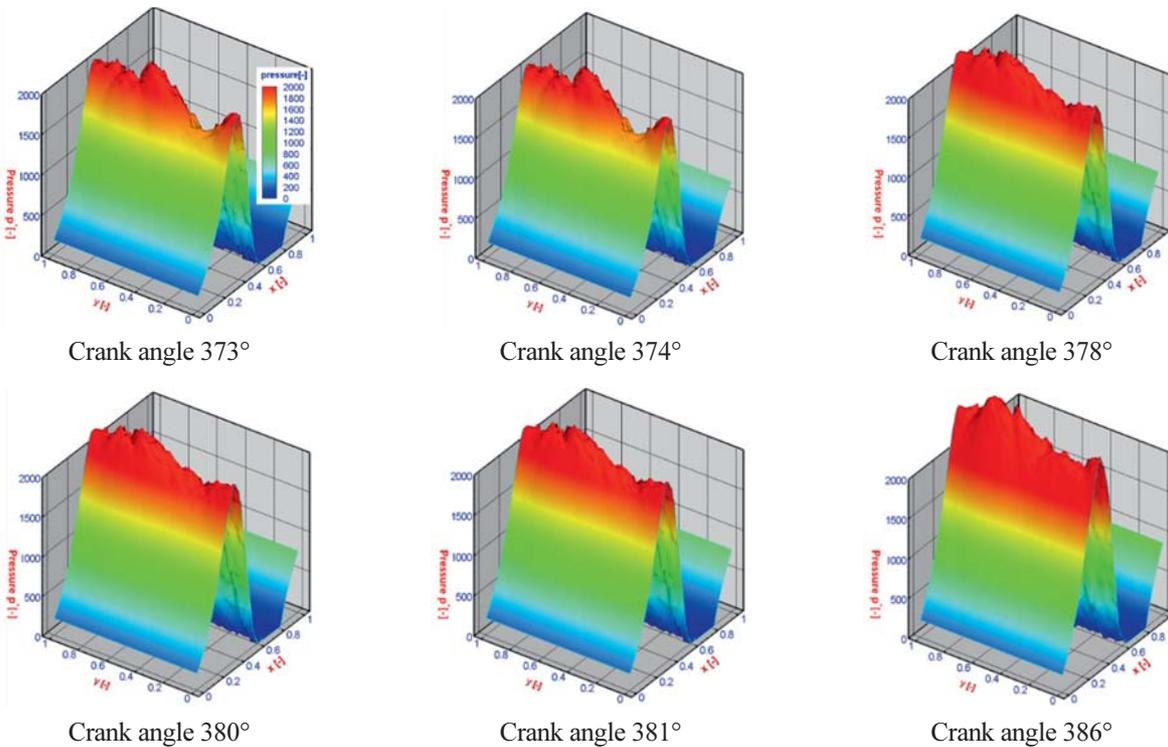
Figure 9. Variations in the hydrodynamic dimensionless lubrication film  $h^* = h/h_{max}$  during a cycle on honing smooth cylinder surface ( $h_{max} = LST \text{ depth} + \text{ honing ridge depth} + R_a$ ) at 3000 rpm under full load.
