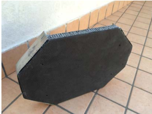
Figure 18. Structure behind the anti-intrusion plate.
