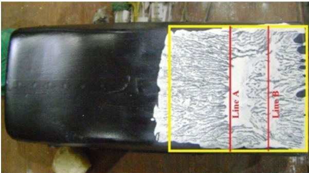
Figure 14. Top view of bare car with oil flow visualization at the rear.
