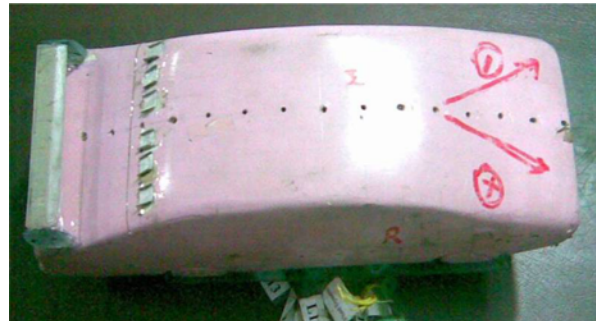
Figure 8. Locations of pressure holes, co-rotating VG array and rear spoiler on the car.
