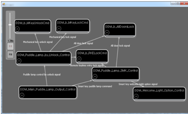
Figure 7. Module flow diagram of a puddle lamp.
