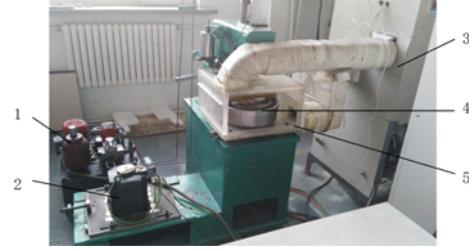
Figure 9. Wear test platform: 1. Hydraulic system; 2. Servo motor drive system; 3. Temperature control unit; 4. Friction turntable; 5. Environmental warehouse.
