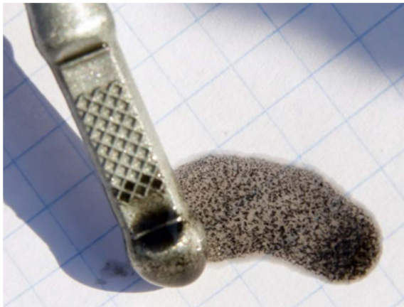
Figure 5. MWCNT in the engine oil, a drop of oil on a piece of paper; oil taken from the sump immediately after stopping the engine; large CNT agglomerates visible (Volkswagen TDI engine, AXD type).
