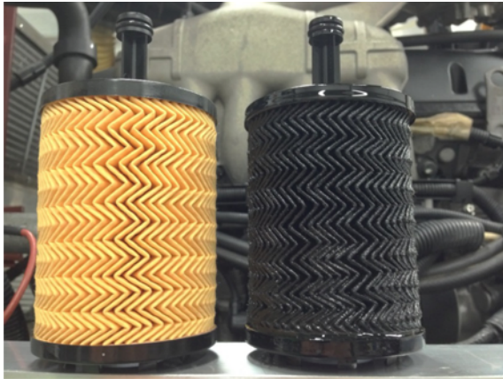
Figure 1. Picture of a new oil filter (left) and an oil filter after two minutes of operation in an engine, with CNT remnants left after previous tests (right).
