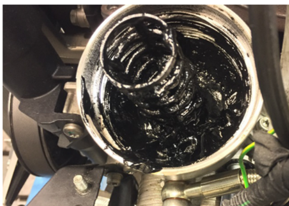
Figure 11. Interior of the oil filter housing after the test with oil containing 1 % MWCNT; oil changed its consistency to resemble stiff grease and was not flowing back from the filter housing to the oil sump.
