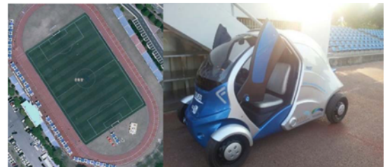
Figure 5. Experimental environment: (a) Test track for driving test; (b) Subject vehicle for testing with two independent motor control at rear wheels.
