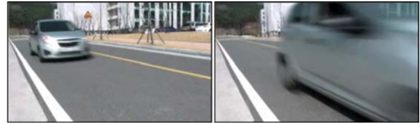
Figure 23. Camera views on a long straight road: When entering the detection area (left), and passing through the BSD zone (right).
