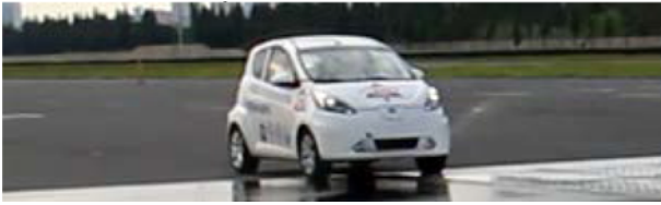
Figure 17. Test on high-low maximum road friction coefficient joint road.
