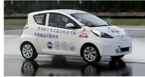
Figure 20. Test on \theta -split road.
