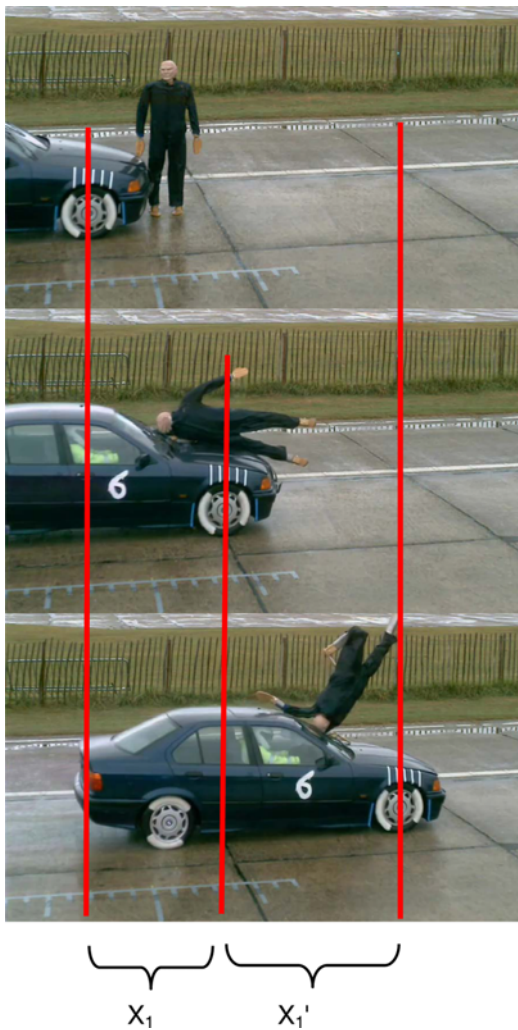
Figure 9. Sub-phases 1.1 and 1.2 – Carrying the pedestrian on hood, test no. 8 (Pedestrian Accident Demonstration, 2013).
