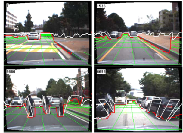
Figure 14. Comparison of free space detection using the proposed algorithm and a laser scanner.
