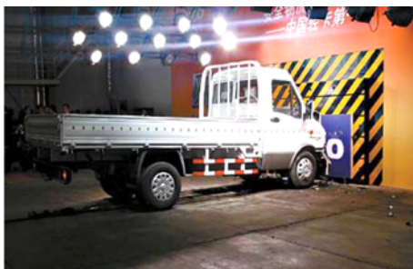
Figure 8. Frontal impact test.
