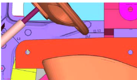
Figure 30. Survival space check of front pillar impact.
