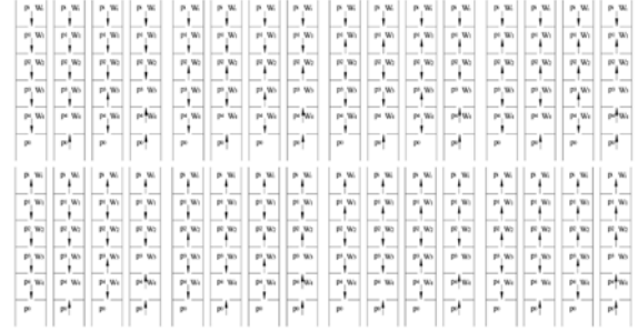
Figure 5. 32 types of blowby patterns among the piston rings.
