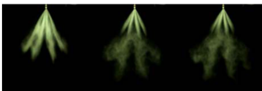
Figure 6. Injector spray visualization for single, double, and triple injection.
