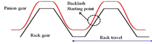
Figure 6. Backlash and starting point of a rack-pinion gear model.
