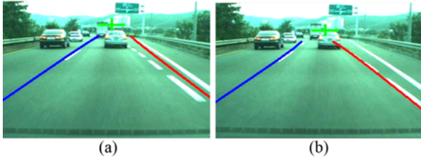
Figure 6. Effect of the representative lane candidate selection. In the case of double right lanes, there can be two representative lane candidates, and the incorrect right lane equation is calculated (a). However, by selecting the nearest candidate, the right lane equation is calculated correctly (b).
