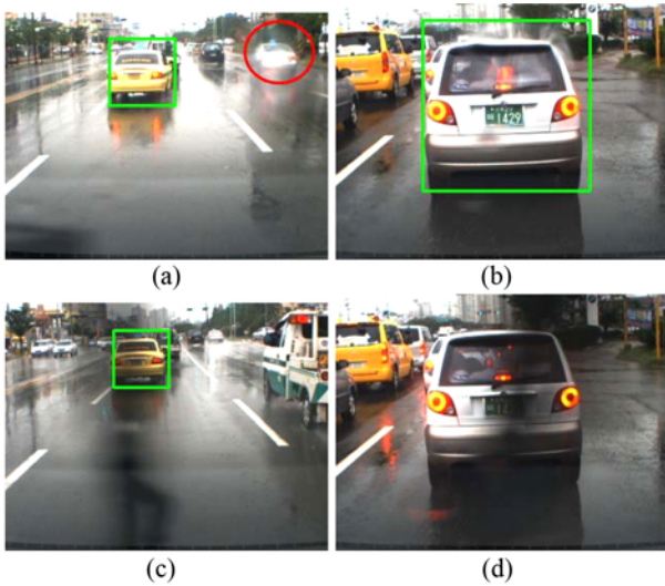
Figure 22. Major factors that degrade the vehicle detection rate on a rainy day: (a, b) distortion caused by raindrops on the front windshield and (c, d) occlusion by the wipers.
