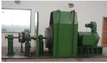
Figure 5. Exclusive test bed for the eddy current retarder.
