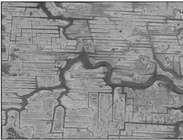
Fig. 9 Extensive grid and parallel ditches that were dug in the 1930s by the Civilian Conservation Corps in Seabrook, NH; darker and wetter areas are seen surrounding ditches in the center and right portions of the photo (Google Earth, photo taken in 2010)
