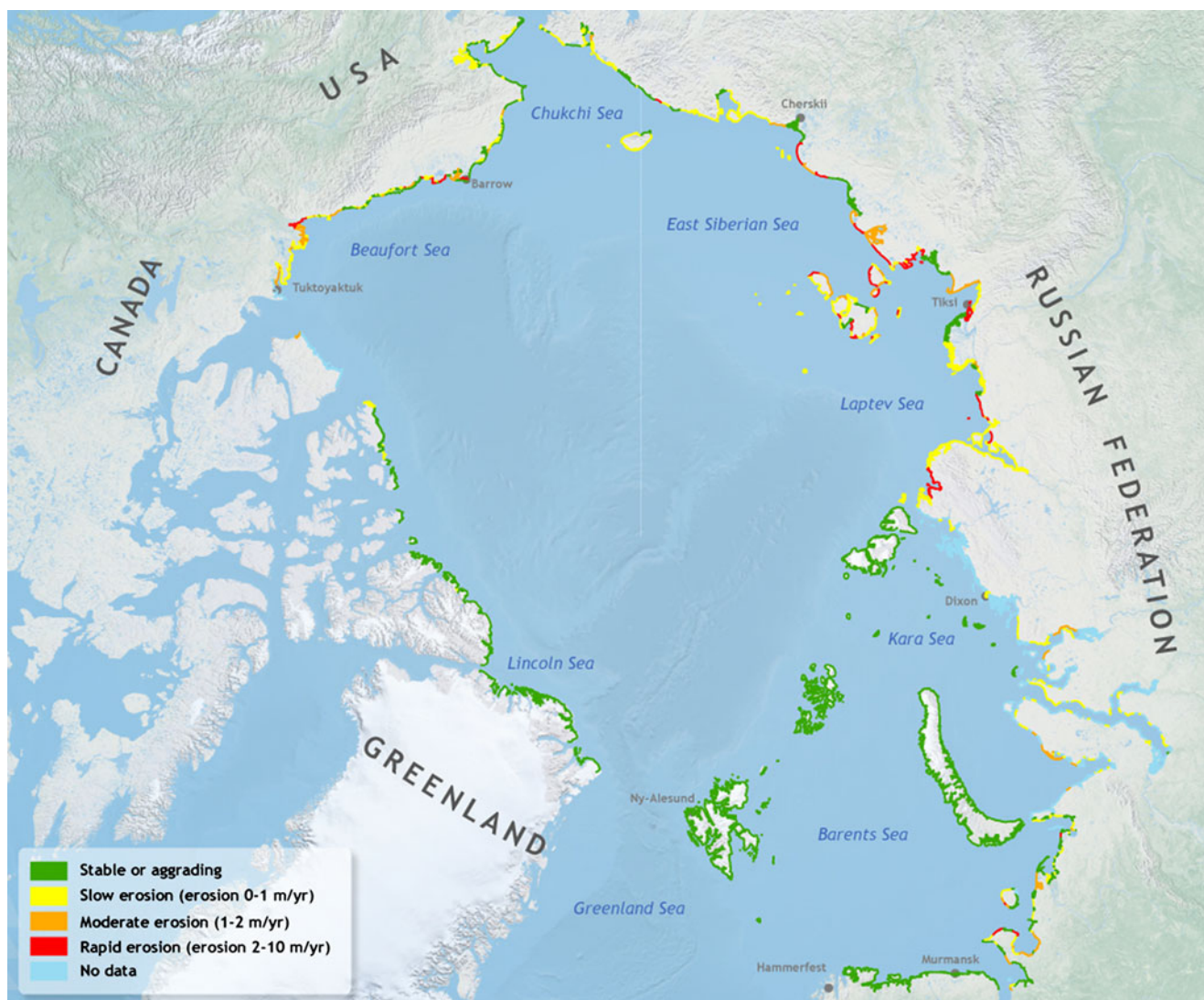
Fig. 6 Circum-Arctic map of coastal erosion rates. The spatial variability in erosion rates generally observed at local scales is also a prominent regional feature
