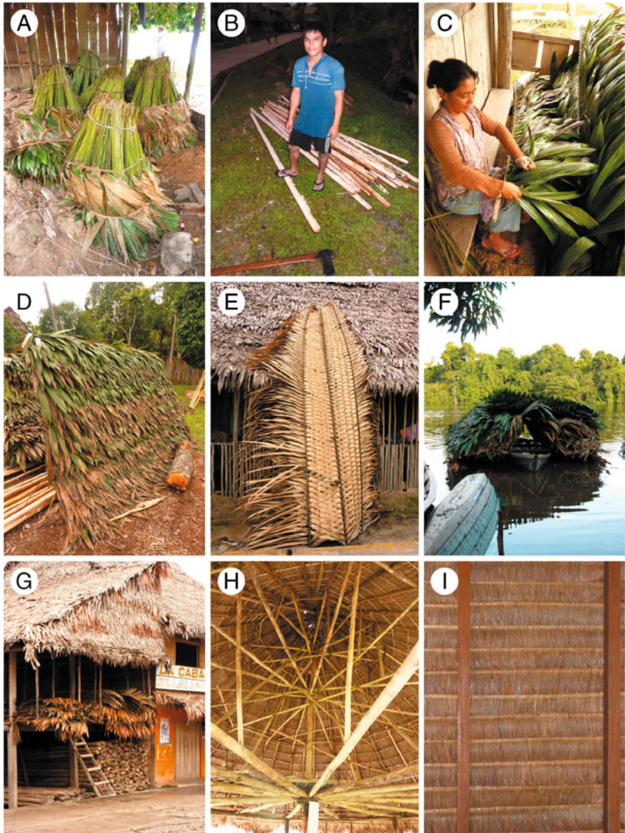
Fig. 2 Use of palm products in construction. a , Lepidocaryum tenue leaf piles ( cargas ) for crisneja production. b , Socratea exorrhiza stem splits ( ripas ) for crisneja production. c , crisneja plaiting. d , stockpiled crisnejas , sales unit el ciento (100). e , roof ridge made of fronds of Attalea spp. f , crisneja transport from producing community to Iquitos (Peru). g , shop for construction materials selling crisnejas in Iquitos. h , palm roof in an indigenous community near Iquitos. i , palm roof made from Geonoma deversa leaves, Parque Nacional de Carrasco (Ecuador). (photographs: a – f , G. Brokamp; g – i , M. Mittelbach)
