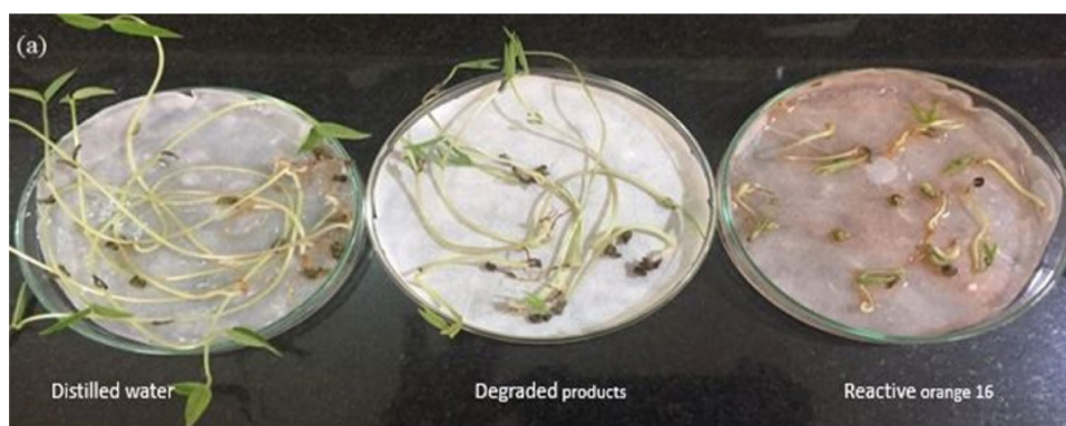
Fig. 9 Toxicity study of dyes (a) reactive orange 16 and its degraded metabolite on germination of Vigna radiata seeds
