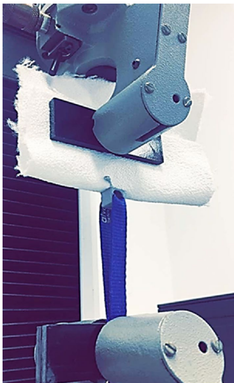
Fig. 4 The tensile test method for 3D printed fabrics
