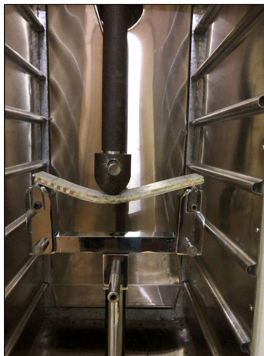
Fig. 5 Photograph depicting the three-point bending test of a fabricated sample
