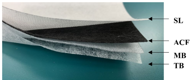
Fig. 1 Cross-sectional image of the composite nonwoven
