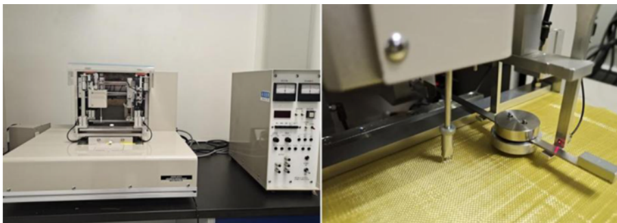
Figure 4. (a) Machine of KES-F4 System and (b) test process of friction coefficient.
