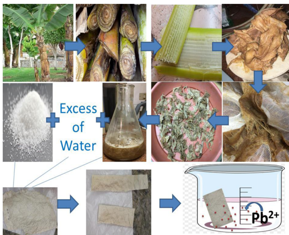
Scheme 1. Illustrated summary of the banana fiber processing as well as films formation and adsorption technique.
